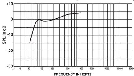
**FIGURE 11 — Maximum SPL at 1 Meter in a Typical Enclosure (1.0 ft<sup>3</sup> tuned to 75 Hz)**
