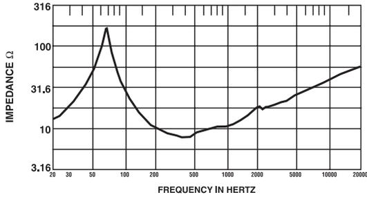
**FIGURE 4 — Impedance in Typical Enclosure (4.0 ft<sup>3</sup>)**
