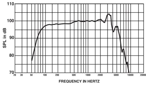
**FIGURE 2 — Frequency Response in Standard Baffle (0° and 45°)**
